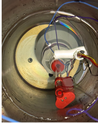
Figure 21: Depth sensor submerged in pressure chamber
