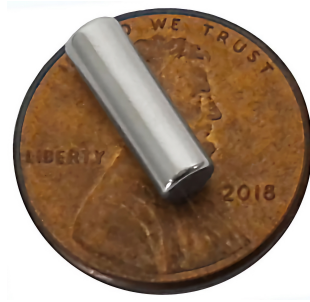
Figure 3: 4 mm x 12 mm N48 cylindrical magnet as used in the magnetic piston. Penny shown for scale
