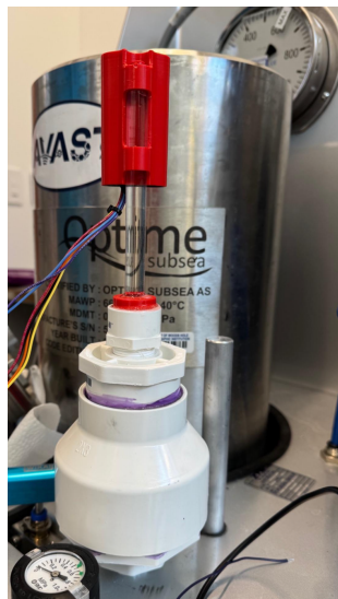
Figure 33: Assembled depth sensor module in front of pressure chamber
